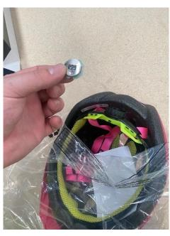
3) Remove the battery & dispose of the light cell.
