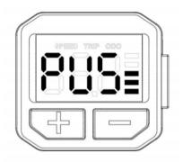
The walk assist feature is not a riding mode. It is designed to assist with walking the bike up an incline to a maximum of 6 kph.
