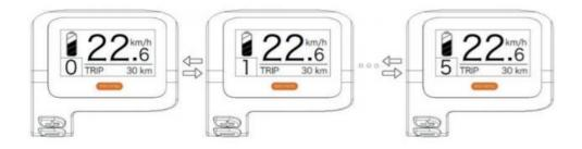
There are 5 pedal assist settings on this bike, level 1 providing the lowest level of assisted power and level 5 the highest. Simply push the plus or minus buttons to change between the levels. Pedal assist does not work in level 0 (zero).
