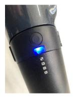
Before riding you may want to check the battery charge by pressing the button on the battery top. The battery charge light will illuminate. The colour of the LED indicates the level of battery charge:
