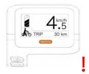
Press and hold the button to engage the Walk Assist function. The kicon will appear in the display and the bike will assist to 6 kph. Release the button to exit the Walk Assist mode.
