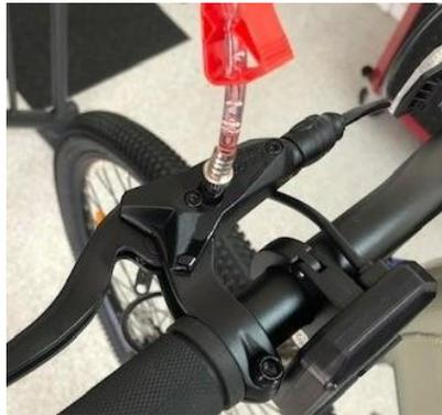
5. Push fluid from the syringe at the caliper until half the fluid volume is in the syringe at the lever
