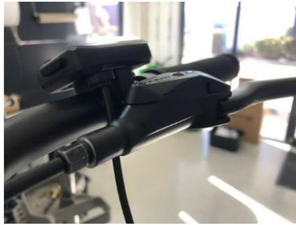
4. Remove the brake lever bleed screw with a T10 Torx wrench and screw in the empty syringe
