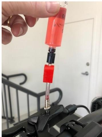
6. Pump both syringes alternatively until no air can be seen coming from the system. It may be helpful to tap the brake hose and caliper gently, and repeatedly with the handle of a screwdriver to shake the air from the system
