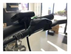
4. Remove the brake lever bleed screw with a T10 Torx wrench and screw in the empty syringe
