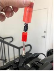
6. Pump both syringes alternatively until no air can be seen coming from the system. It may be helpful to tap the brake hose and caliper gently, and repeatedly with the handle of a screwdriver to shake the air from the system
