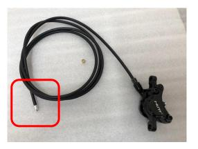
• When the homing head is removed the treaded insert serves as the needle and only a new olive is required on the hose. The threaded insert does not need to be replaced with a new needle
