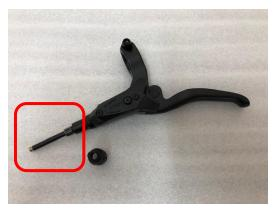
• The caliper hose is fitted with a "homing head" to contain the fluid and assist in running the hose through the bike frame
