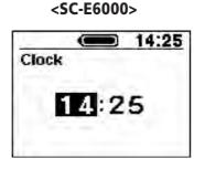
4. Press the Assist-X or Assist-Y to set the minutes, then press the Assist-A enables the set value. The "Setting menu" screen is displayed.
