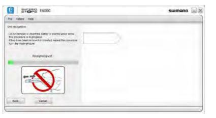
4. Invokes the unit with the corrupted firmware, and overwrites its firmware with new firmware.
