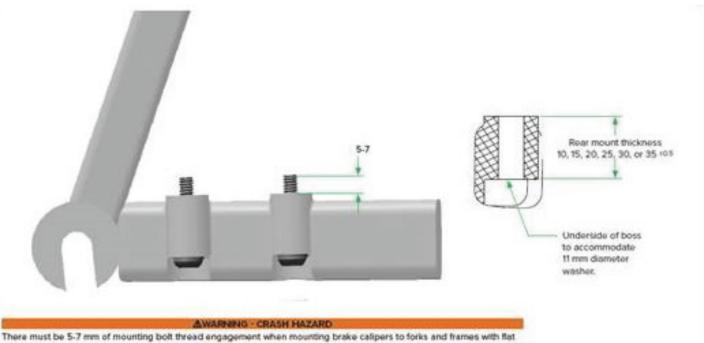
There must be 5-7 mm of mounting bolt thread engagement when mounting brake calipers to forks and frames with flat mount hardward and brackets. Riding a bike with improper bolt engagement can allow the brakes to disengage from the bicycle, which can lead to a crash and serious injury or death to the rider.
