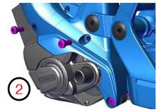
3. Carefully flip drive unit down. Watch for those electrical wired to not get pulled off! (image 3)
