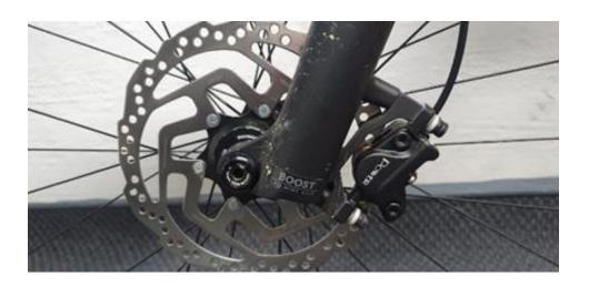
This decision to use the POWER brakes was based on availability as the earliest delivery from SHIMANO or TEKTRO was OCT 2022. Effectively meaning we wouldn't have any stock until November 2022. Testing by our design team in Germany showed that the performance was comparable to the Shimano MT200 brakes and all braking distances (wet and dry) were way shorter than required by ISO 4210.
