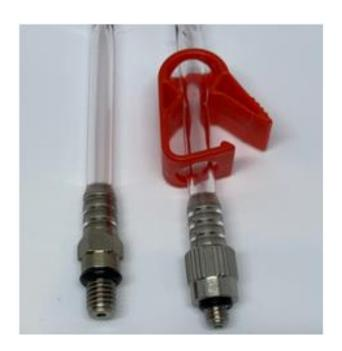
These are the two connectors to look out for. The lock is on the connection that goes onto the brake lever.
