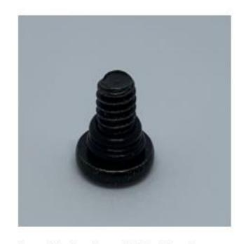
Lever bleed port cap (t10 tool) has 2 O-rings. Be sure both come out before attempting to bleed system. Use an O-ring pick (BZBM20ORINGP) if they're proving tricky
