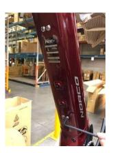
Locate wires at top-side of downtube and pull out and away from under battery bracket.
