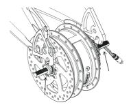
5. Mount the 4mm washer on both sides of the frame.
