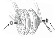
7. Mount the shaft end sheath (M12 flange nuts) on both sides of the shaft ends.
