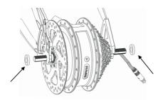
6. Tighten the M12 flange nuts with open spanner at both sides of the motor. (torque requirement: 47-60N.m.)
