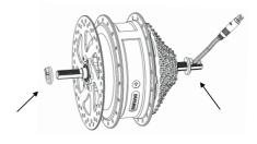
4. Insert the motor into the frame.
