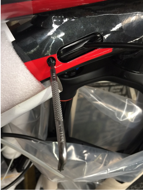
Step 1 - remove T10 screw
