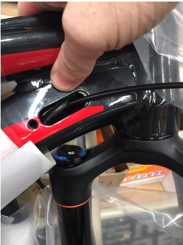
Step 3 - feed cable plate out through access hole
