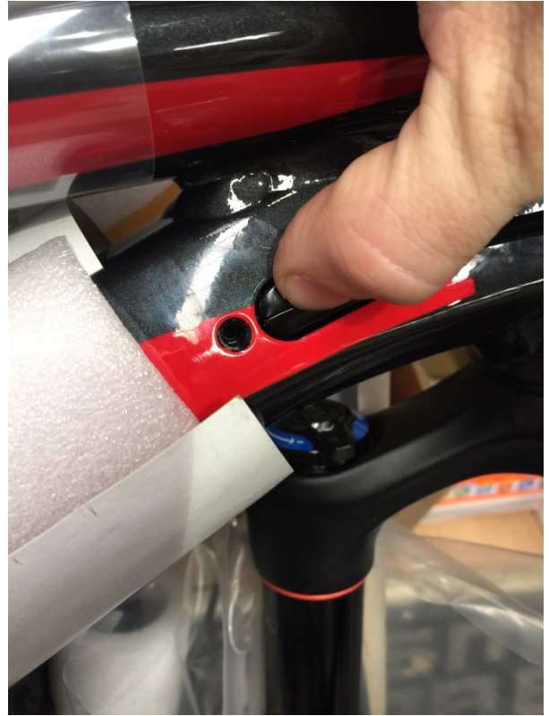
Step 2 - Push plate into downtube
