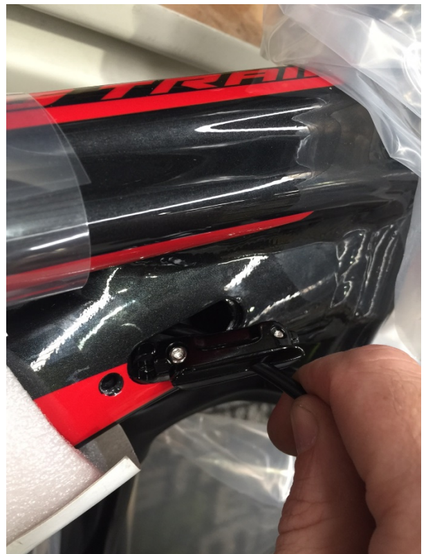
Step 4 - loosen two plate bolts
