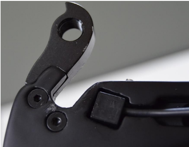
The distance between the sensor and the locking should not be below 3mm
