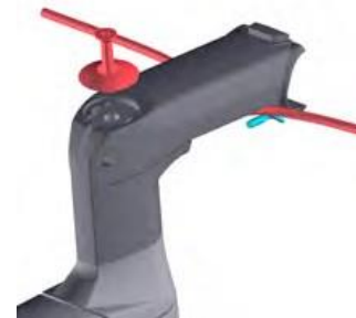
Install top cap and compression bolt
