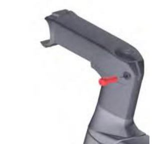
Install stem steerer clamp bolt - grease required!
