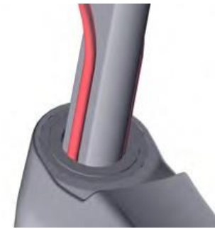
Install bearings and compression ring – cables will sit securely on flat sides of steerertube
