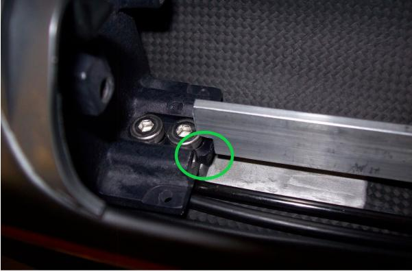
8. Once the distance is set tighten the two screws #1 with a 4mm torque wrench to 6Nm then reinstall the upper latch using a 3mm torque wrench to tighten the four screws as shown below
