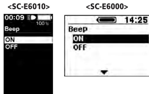
4. Pressing the Assist-A button enables the set value at the cursor position. The "Setting menu" screen is displayed.
