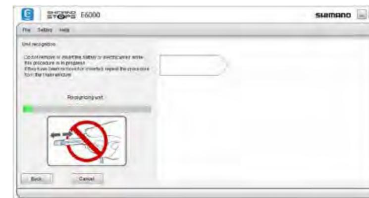
4. Invokes the unit with the corrupted firmware, and overwrites its firmware with new firmware. Click "Next".
