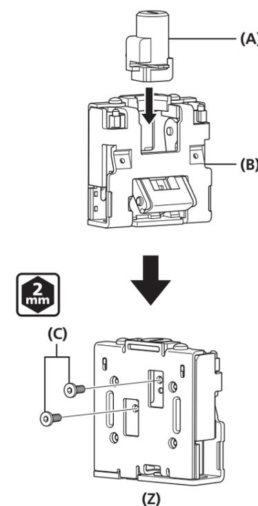
5. Align the fixing bolt holes in the key unit with the frame mounting holes.
