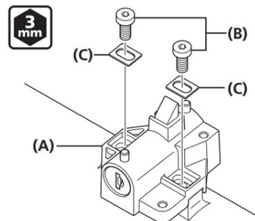
4. Adjust the position of the key unit so that the distance between section (A) of the key unit and section (B) of the mount lower case is 224.4mm and then fully tighten the key unit fixing bolts.
