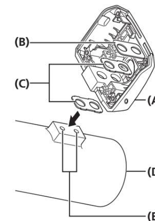
2. Secure the mount lower case by tightening the two types of mount fixing bolt (M5). Tighten the mount fixing bolt (M5) (low head type) first.
