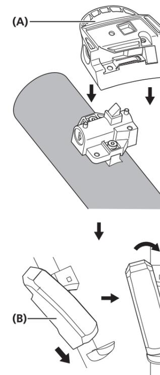
6. Secure the key unit cover with the key unit cover fixing bolts (M4).
