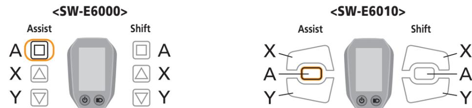
5. Press the Assist-X or Assist-Y to move the cursor to "Exit".
