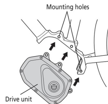
2. Insert M8 bolts, attach nuts from the opposite side, and tighten them to the designated torque.
