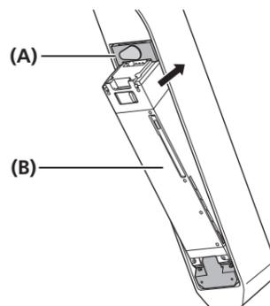
Attaching/detaching the battery on downward attachment/removal design frames
