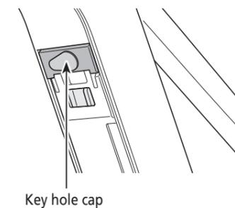
**2. Insert the key into the key cylinder in the battery mount.**
