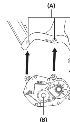
2. First attach the drive unit fixing bolts (M8) to the right side. After this, attach the drive unit fixing bolts (M8) to the left side. Tighten the drive unit fixing bolts (M8) until the drive unit makes firm contact with the inside of the right side of the frame.
