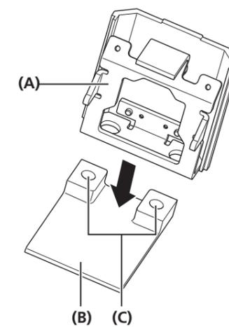
2. Secure the mount lower case to the frame by the tightening the mount fixing bolts (M8).
