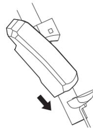
2. Slide the battery to the right starting from the point where it is inserted. Push in the battery until you hear it click.
