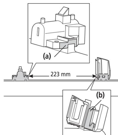
6. Fully tighten the key unit cover fixing bolts (M4) to attach the key unit cover.
