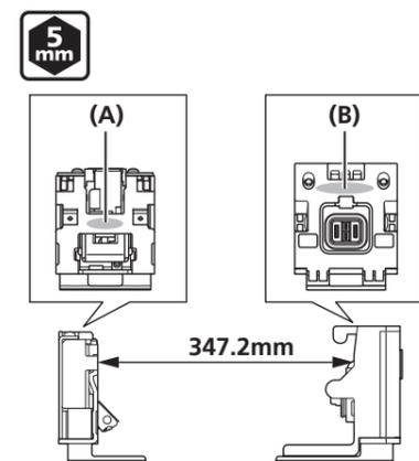
7. Temporarily attach the key unit cover to the key unit and adjust so that the battery can be smoothly connected/disconnected and no noise is produced due to looseness during riding.
