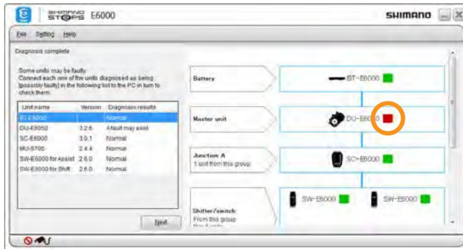
4. If a malfunction might occur, recheck using a single connection.
