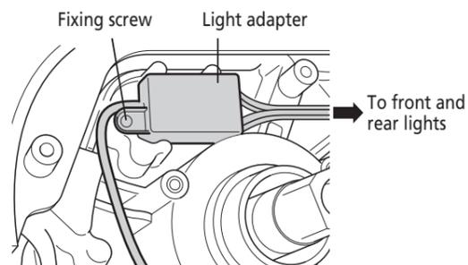
3. Remove the dummy plug from the drive unit with Shimano original tool <TL-EW02>.
