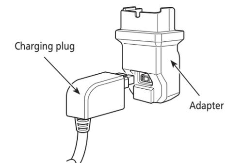
6. Attach the adapter (<EC-E6000>) / charging plug (<SM-BCE60>) into the charging port.
