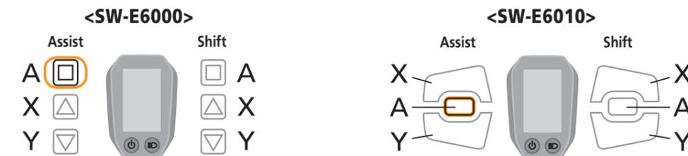
5. Press the Assist-X or Assist-Y button to move the cursor to "Exit".
