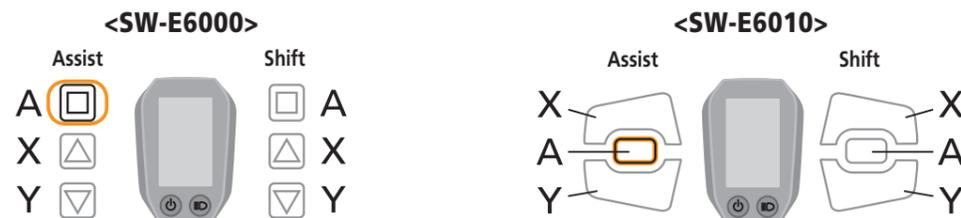
5. Press the Assist-X or Assist-Y to move the cursor to "Exit".
