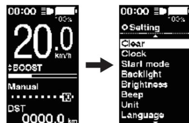
2. Press X or Y to select the various menus. Press A to display the setting screen for the selected menu.
