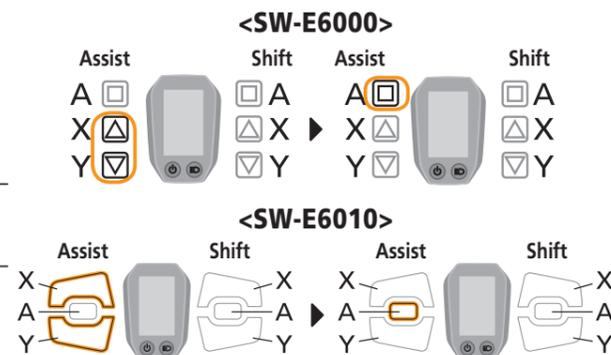
5. Press the Assist-X or Assist-Y to move the cursor to "Exit".
