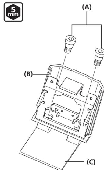
3. Route the battery cable through the cable routing hole in the mount lower case and then tighten on the mount upper case using the mount upper case fixing bolts (M3).
