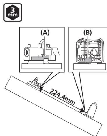
5. Temporarily attach the key unit cover to the key unit and adjust so that the battery can be smoothly connected/disconnected and no noise is produced due to looseness during riding.
