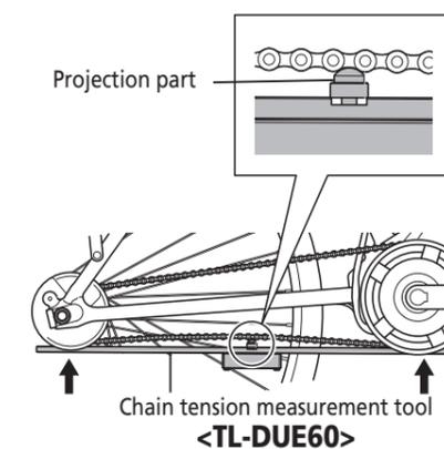
3. Adjust the chain tension so that part C of the projection part is not hidden by the chain tension measurement tool's frame.
