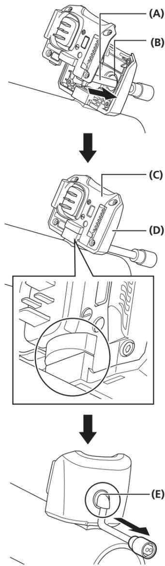
8. Tighten on the mount upper case using the mount upper case fixing bolts (M3).
