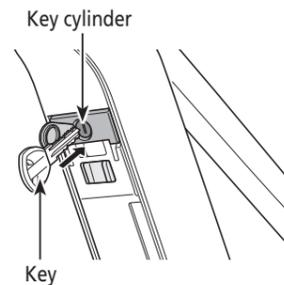
**3. To unlock the battery, turn the key clockwise and push it in.**
