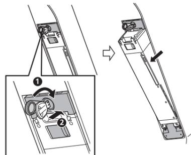
**4. Remove the key from the key cylinder, close the keyhole cap, and detach the battery.**
