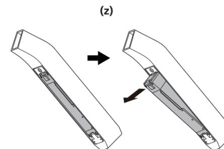
(z) Downward attachment/removal design frame
