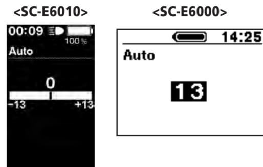
4. Pressing the Assist-A button enables the set value at the cursor position.
