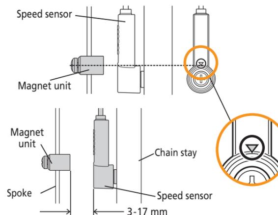
2. Before installing the speed sensor, check that the clearance between the speed sensor and the magnet unit will be within 3 to 17 mm.
