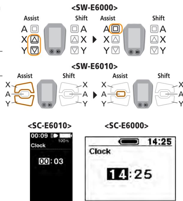
4. Press the Assist-X or Assist-Y to set the minutes, then press the Assist-A enables the set value.
