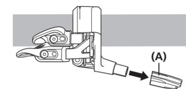
2. Pass the electric wire through the cable cap, and connect it to the assist switch.
