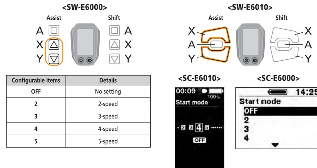
4. Pressing the Assist-A button enables the set value at the cursor position.
