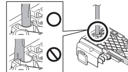
3. Mount the lower case sub assembly and the battery mount rail using the M4 bolt (C).
